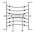
(ii) The behaviour of magnetic field lines in the presence of a diamagnetic substance is shown :
