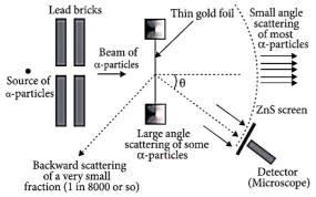
Schematic arrangement of the Geiger-Marsden experiment
