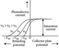
Einstein's photoelectric equation: If a light of frequency  $\upsilon$  is incident on a photosensitive material having work function  $(\phi_0)$ , then maximum kinetic energy of the emitted electron is given as
