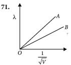
(i) In terms of accelerating potential V, the de Broglie wavelength of a charged particle is given by
